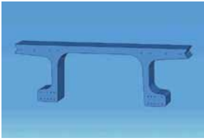
The UHPC Pi Girder is a 33-in.-deep and 100-in.-wide decked bridge girder designed to span up to 87 ft and allows for rapid construction of an extremely durable superstructure.
